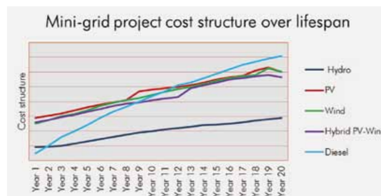
Figure 1: Costs associated to a mini-grid over its lifespan.
